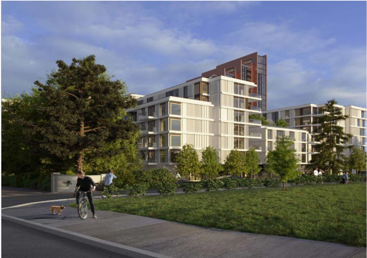
Figure 5.8: View of the scheme from Golf Lane, the scale and height of development steps down to avoid overbearing and amenity impact on the adjacent properties along Golf Lane
